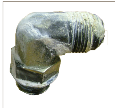
Figure 5: Zinc Oxidation on a Steel Tube Fitting
